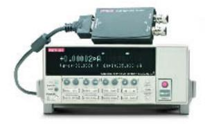
The **Model 6430 Sub-Femtoamp Remote SourceMeter** combines voltage and current sourcing and measurement capabilities with sensitivity, noise, and input resistance specifications superior to electrometers. On its 1pA range, it can measure currents with just 0.4fA p-p noise for applications like characterizing the conductivity of polymers and single electron transistors (SETs).
